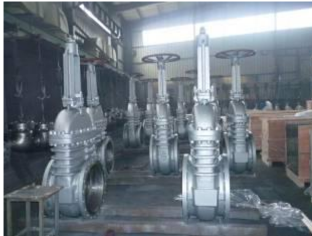
Gate Valve under the Silver Grey Painting process
