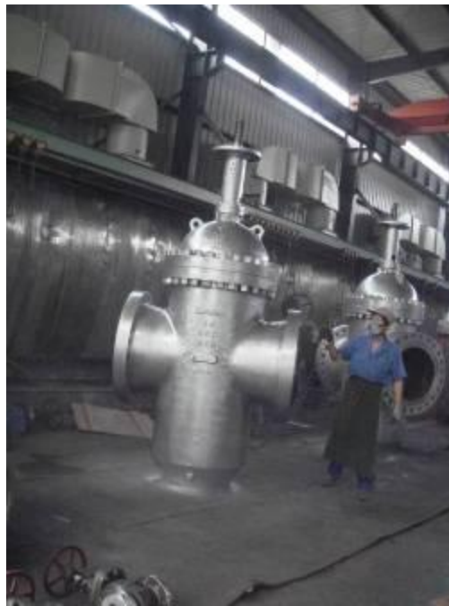
Through Conduit Gate Valve
